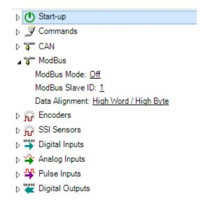
From the configuration you could set Modbus mode to (Off, TCP, RTU over TCP, RS232 ASCII, RS485 ASCII, RS232 RTU or RS485 RTU). You will be also able to set the Modbus Slave ID as long as the desired data alignment.
