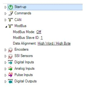
From the configuration you could set Modbus mode to (Off, TCP, RTU over TCP, RS232 ASCII, or RS485 ASCII). You will be also able to set the Modbus Slave ID as long as the desired data alignment.
