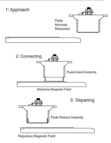
FIGURE 5. Collector pads extension and retraction depending on position over base
