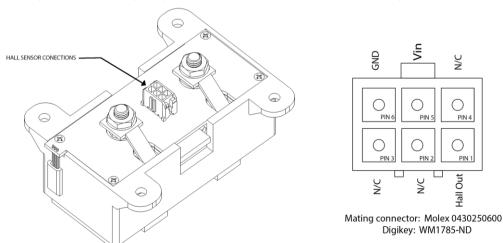
FIGURE 11. Connection to the Hall Sensor
