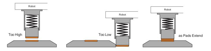
FIGURE 6. Spring loaded pads have lower ground clearance and must be adjusted tight height tolerance
