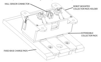
FIGURE 1. RoboPads Charge System composition
