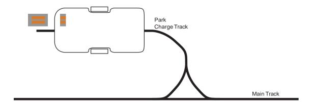
FIGURE 4. Charge pads located at charge parking
