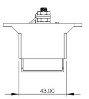
FIGURE 14. Collector charge pads mechanical dimensions
