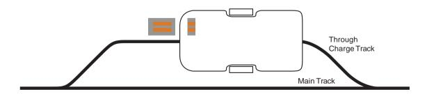
FIGURE 3. Charge pads located at diverted track
