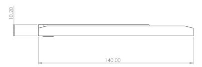
FIGURE 13. Base charge pads mechanical dimensions
