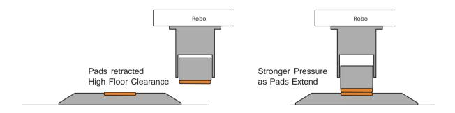
FIGURE 7. RoboPads have higher floor clearance and much stronger contact pressure
